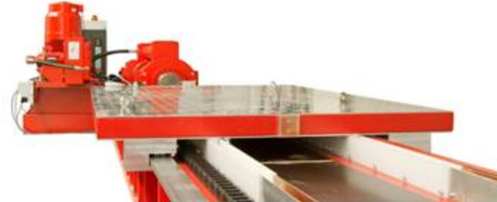
Testing seats, seat belts, whiplash and other components
