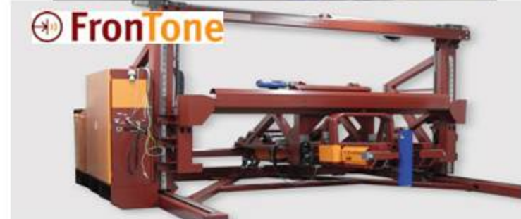
Testing seats, seat belts, whiplash and other components
